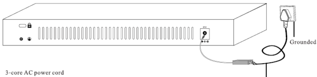
Figure 2.7 Ground with 3-core AC power cord
