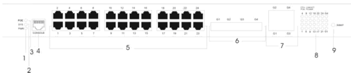
Figure 1-1 Front template of the ST-POE24M switch
