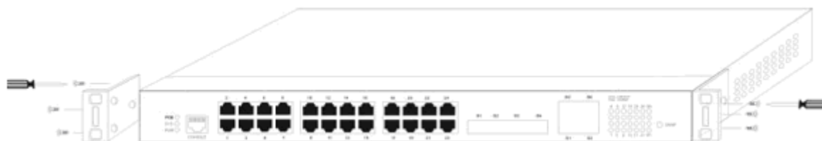
Figure 3-1 Fixing the machine box of the switch
