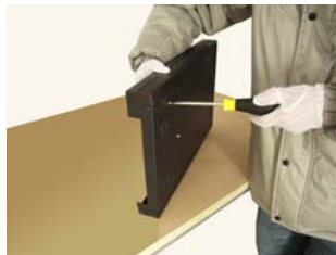
Install the HDD screws
