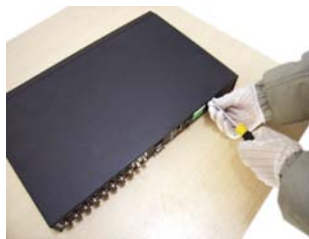
Remove all cover screws
