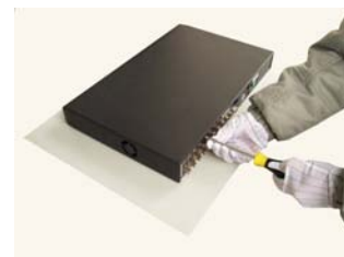
Reinstall the cover screws
