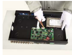
Connect the power cable
