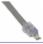
This ezEX<sup>™</sup>44 connector is designed for larger cables and conductors. Features a unique integrated Hi-Lo stagger load bar and allows 'big' conductors to pass through the front end of the connector making it easy to verify the wiring sequence before terminating. This connector is typically used with Cat6 and is terminated with EXO Crimp Frame® and EXO-EX Die<sup>™</sup> (100061C). Cat-5e/6/6A compliant, works with solid or stranded 24-22 AWG conductors
