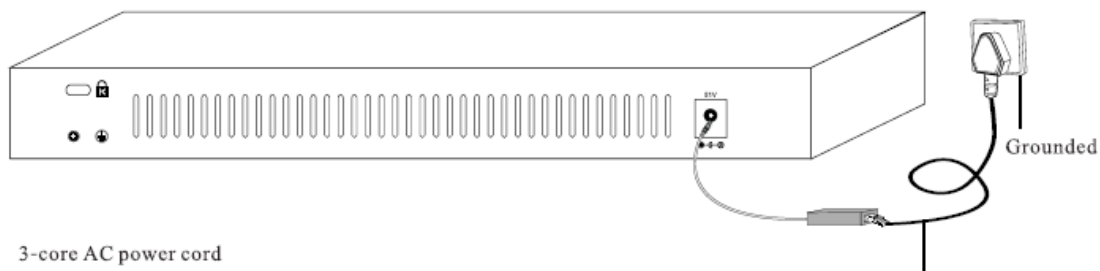
Figure 2.7 Ground with 3-core AC power cord
