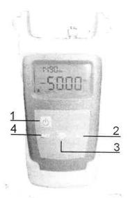
(1) "Power Supply Switch: Press it to turn on or off the unit
