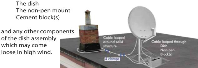
After passing the cable through all above items, bring the end of the cable back to form a loop. Use 2 of the 4 cable clamps to clamp the end of the cable to the main run of cable:
