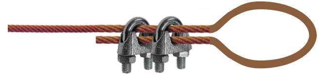
Once the dish is secured to one end of the cable, pass the other end around a solid structural element on the roof, which will be capable of holding the dish is high wind. Create a loop around the structure (chimney, beam, railings, etc) and secure the loop with the other 2 clamps provided in the kit.
