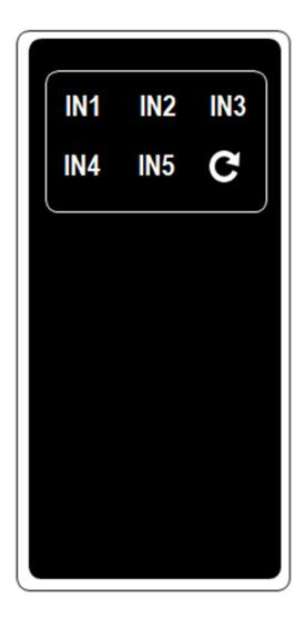
**IN1/IN2/IN3/IN4/IN5:** Press IN1/IN2/IN3/IN4/IN5 button to switch HDMI source signal to output display, and the corresponding LED will illuminate.
