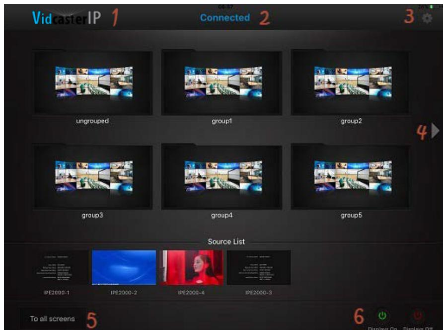
When VidCasterIP is connected to the DT-HDVD-IPSTR-CB, the main screen above is displayed. For more information, see the table below.
