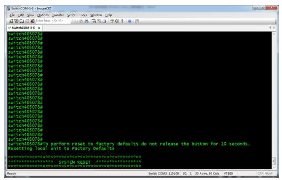
The prompt above means that switch is reset to factory defaults and starts rebooting. Now you can release Reset button and wait until switch finishes rebooting, and then operate based on the previous step 3.
