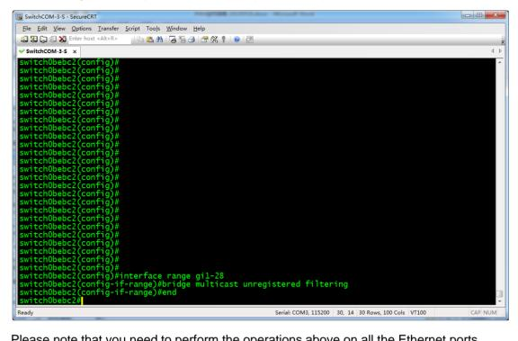
Please note that you need to perform the operations above on all the Ethernet ports connected in the network. If other ports are used, configure them according to the example above.
