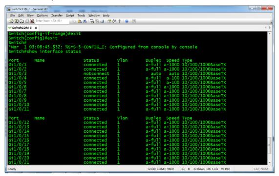
From the figure above, Gi1/0/4 port speed is changed to 100Mbps.
