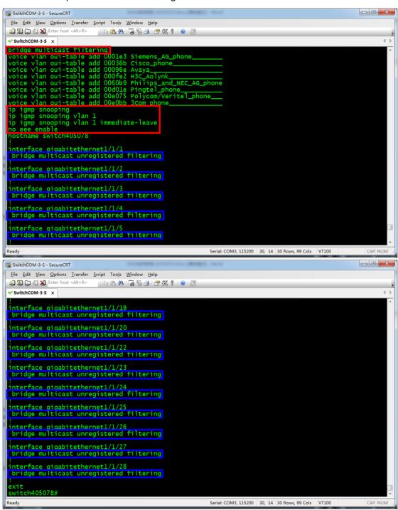
Five configuration commands are marked in red boxes. The commands marked in blue boxes are set on each port configuration except on port 21. If your confirmation result is the same as above, it indicates that SG500 series switches are correctly configured.
