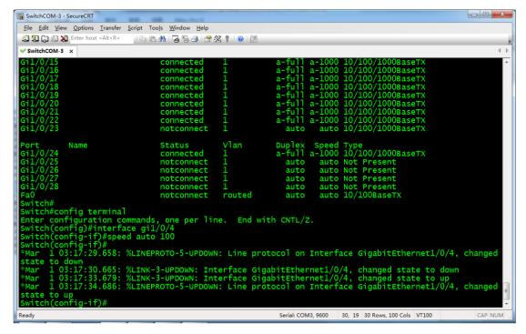
You can also use **interface range** command to assign multiple successive ports for bulk mode change.
