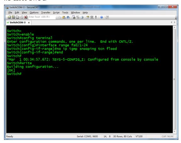
Now, multicast flooding caused by TCN has been successfully prevented from all host ports. Please note that in the previous example we only configure main ports of switches except a few ports such as WS-C2960-24TC-L's two Gi ports. You can configure these undone ports according to the example above.
