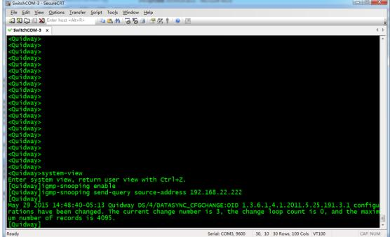
4. In system view input **vlan 1** to enter the view of VLAN 1.
