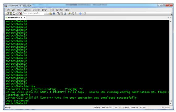
Now, the confirmed configuration is saved. Switch will continue to run the configuration for the next startup.
