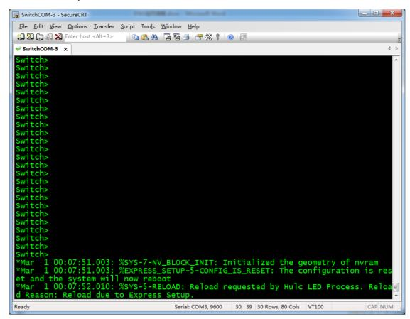
The prompt above means that switch is reset and starts rebooting. Now, you can release **MODE** button. Wait until switch finishes rebooting and follow the instructions in step 4.
