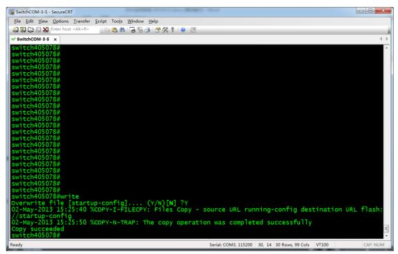
Now, the confirmed configuration is saved. Switch will continue to run this configuration for the next startup.
