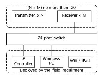
The illustration above is a topology of a single 24-port switch networking. You can choose a switch from the following.
