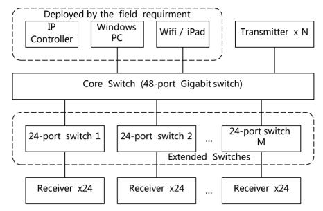
In most cases, it will not require too many TX for networking and all TX can be centrally deployed. You can use them for networking based on the illustration above.
