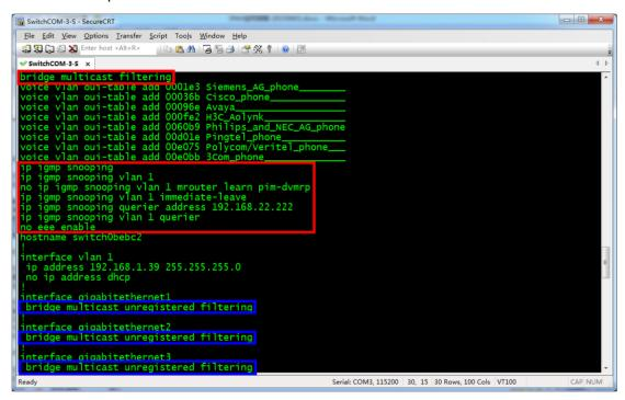
Eight configuration commands are marked in red boxes. The commands marked in blue boxes are set on each port configuration. If your confirmation result is the same as above, it indicates that SG300 series switches are correctly configured.
