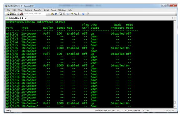
Parameters in speed column are the port speeds. "100" means 100Mbps. "1000" means 1000Mbps.
