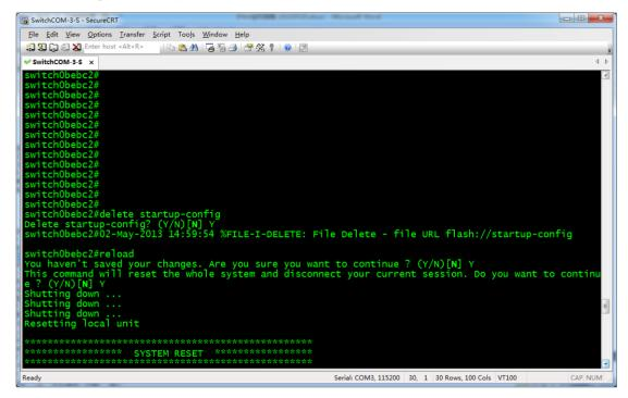
Switch reboots. When the following prompt appears, quickly press Enter twice to complete the baud-rate detection process.
