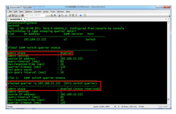
Continue to input **show ip igmp snooping detail** to view IGMP Snooping detail.
