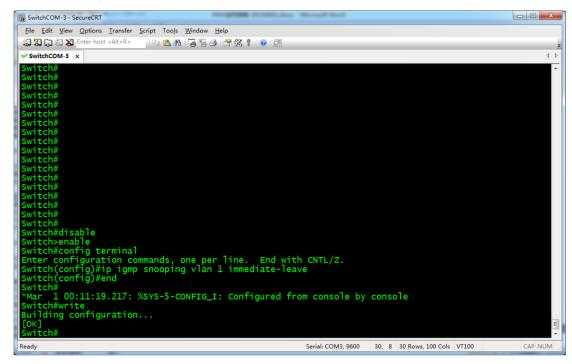
Now, C2960 series switches have been successfully configured to be extended switches.
