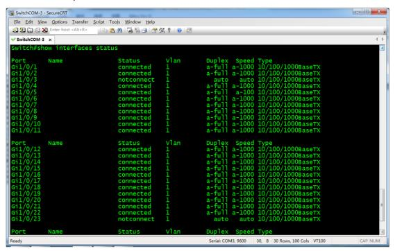
Parameters in speed column are the port speeds. "100" means 100Mbps.
