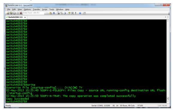
Now, the configuration is saved. Switch will continue to run the configuration for the next startup.
