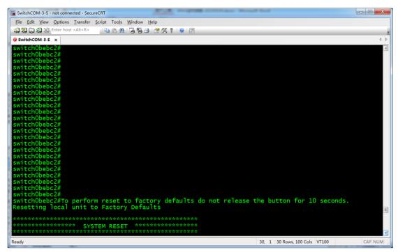
The prompt above means that switch is reset to factory defaults and starts rebooting. Now you can release Reset button and wait until switch finishes rebooting and then operate based on step 3 above.
